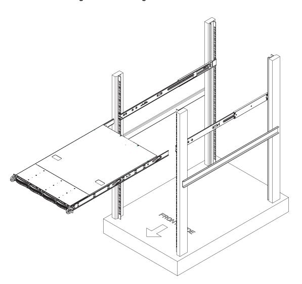
Figure 2-3. Installing the Server into a Rack
